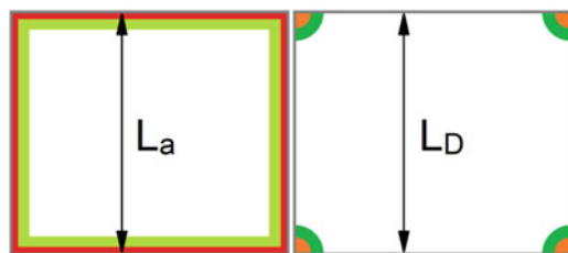
Fig. 5.2 A square network of zero-dimensional (0D, right) and one-dimensional (1D, left) defects enclosing a crystalline area (white) with similar structural parameters L_a = L_D , where L_a is the distance between line-defects (or the crystallite size) and L_D is the distance between point-defects
